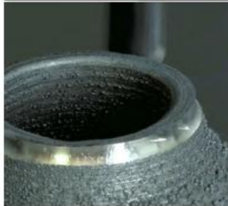
Subtractive Process (Milling) : 155 min
