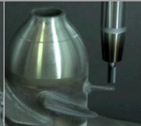
Subtractive Process (Milling) : 155 min
