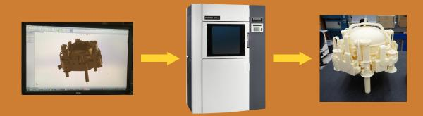
Digital printing and related technologies enable rapid iterations from concept to hardware prototype and even production.
