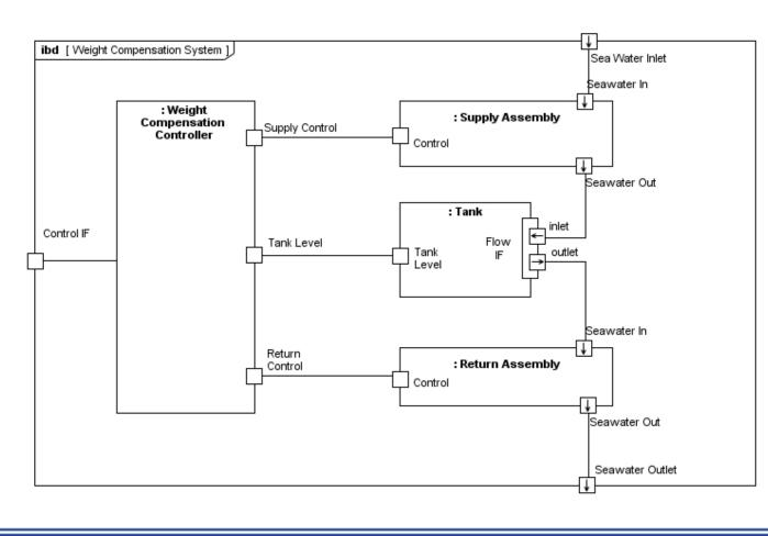
Very abstract (no mention of pumps or valves yet), but still some solution involved: i.e. seawater used to adjust buoyancy via a tank (could have said 'storage assembly')
