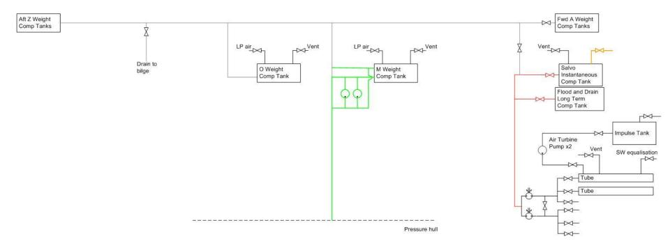
More detail – 'secondary' functions included e.g. drain & vent, recirculation loop for pumps, multiple tanks, interconnects with other systems
