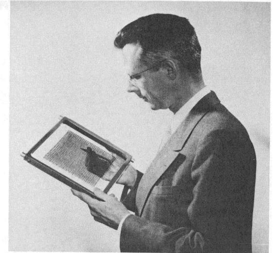
Forrester with a 64 by 64 core memory plane.
