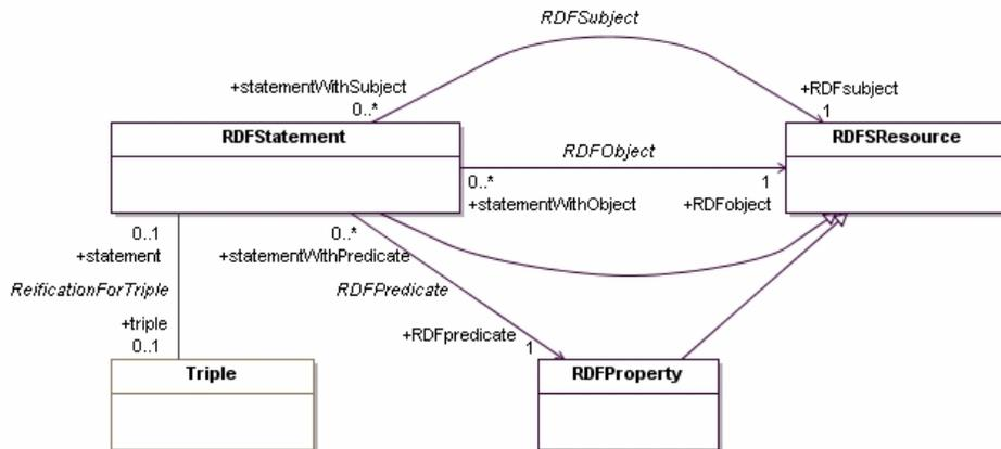
Figure 10.? – RDFBase Package, The Reification Diagram
