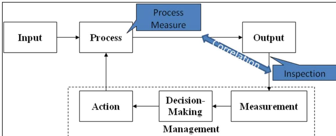
Figure 1. Measurement model as a closed-loop feedback control system for management.
