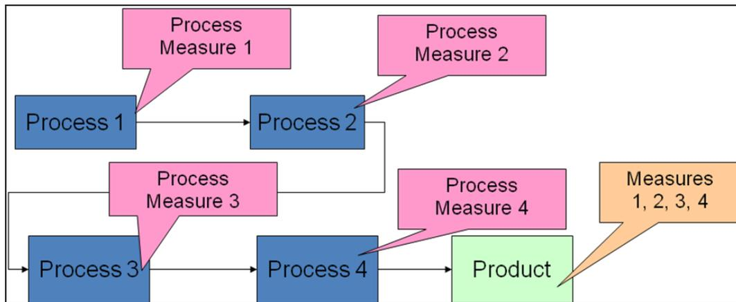
Figure 3. Example process measures for each process step need to be correlated with product measures.
