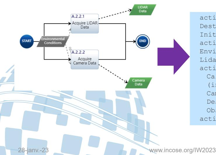
action def Drive Vehicle (in Destination Location : data, in Initial Location : data); action def Monitor Environment (in Environmental conditions : data, out Lidar data : data); action def Calculate Waypoint and Obstacles (in LIDAR data : data, in Camera data : data, in Destination Location : data, out Obstacles : data); action def Navigate Vehicle;
