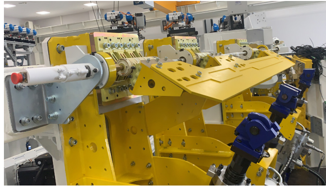
Figure 39. Control surface, aircraft actuator, and loading actuator installed on the Iron Bird
