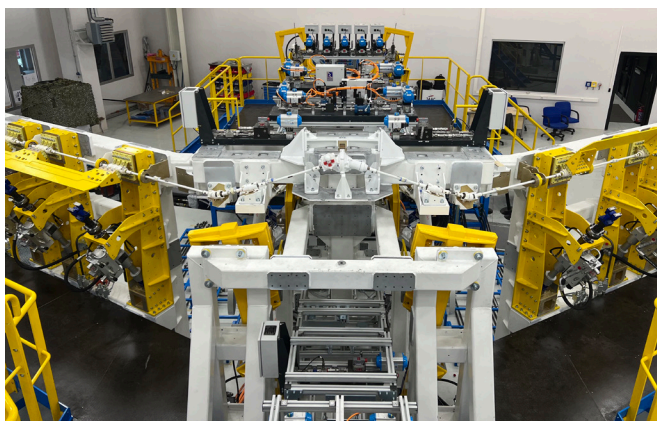
Figure 37. General Structure of an Iron Bird
