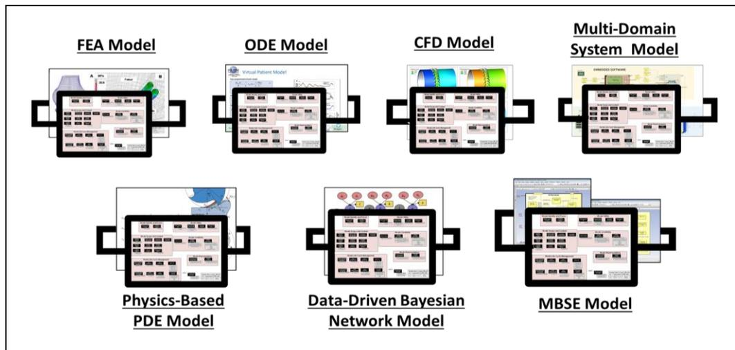
When the information characterizing a specific virtual model is inserted into the generic MCP's data structure, the result is referred to as a "configured MCP", because it now describes a specific virtual model. The configured MCP is sometimes also referred to as a "Model Wrapper", because it is in many ways analogous to the printed labels and bar codes that are found on packaged food products on a grocery shelf.
