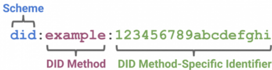
Figure 1: A simple example of a decentralized identifier (DID) (From the W3C)
