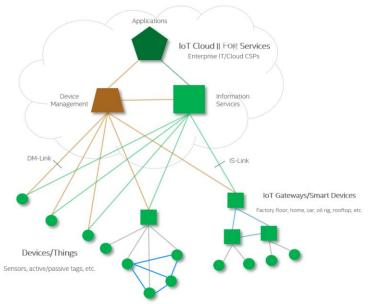
There are many possible interactions/links between the IoT elements. We are focusing this discussion on two important interactions as denoted in the diagram as Device Management (DM)-Link and Information Services (IS)-Link.
